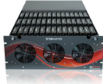
S45 45 HDD Bays
